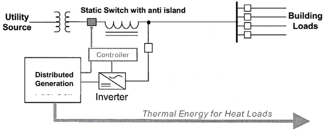
**Figure 4.2 CHP System with Power Quality Functionality**
