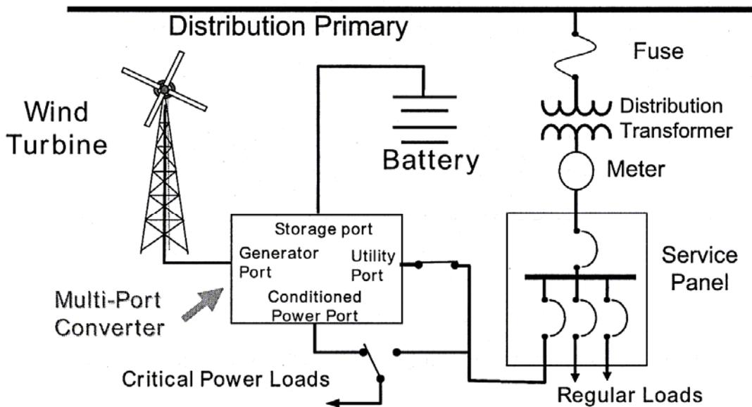
Figure 2.6 Use of Intermittent DG within PQ Environment (Wind)
