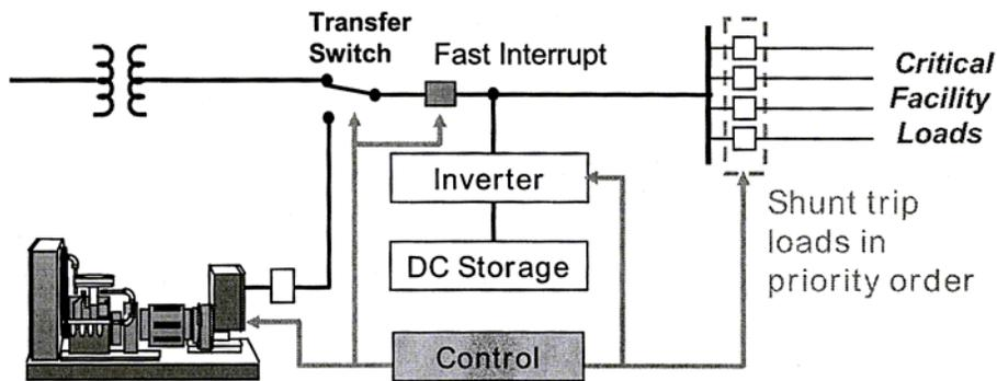
**Figure 4.1 Typical System for PQ and Reliability Support**
