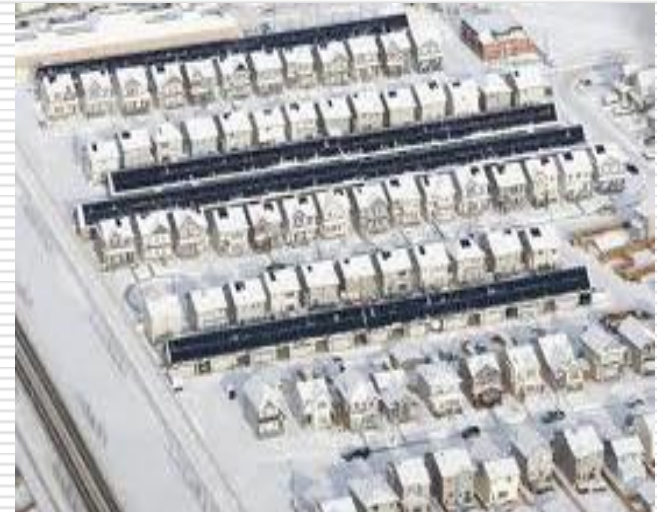
Drakes Landing, Okotoks, Alberta, Canada Solar Thermal Provides 90% of Space Heating (Alberta has 5,199 Heating Degree Days/Year)
